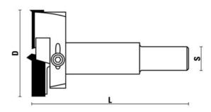
Forstner bore with cylindrical shank and adjustable diameter (60mm-80mm) for boring of concealed hinges in most types of wood or panels. This high quality hinge boring bit has two Tungsten cutting edges, two Tungsten spurs and a HW center point for boring with the best quality on every kind of wood or panels. Right hand boring only
