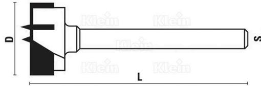
Forstner drill bit with cylindrical shank for boring hinges with the best quality on every kind of wood or panels. This high quality hinge boring bit has two Tungsten cutting edges, two Tungsten spurs and a HW center point for boring with the best quality on every kind of wood or panels. Right hand boring only
