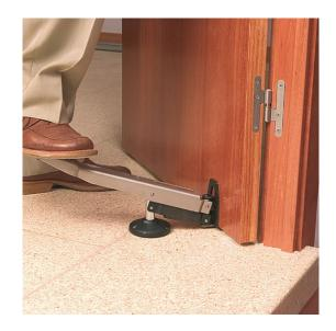
Easy and safe lifting of door panels, furniture, ... This door lift has a loading capacity of up to 200 kg. Equipped with swivel base and anti-slip surface. Made from aluminum. Maximum lifting height 75cm.
