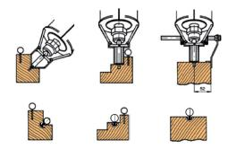
Double 'anchor' bit to be used on the Virutex RA17VG slotting machine. This milling cutter makes it possible to mill in silicone seals type FS2 or FS4.
