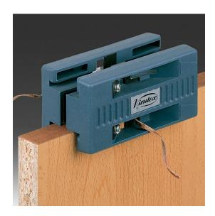
Double edge trimmer for simultaneous trimming of edges up to 40 mm. For wider edges, use as two different trimmers. High-quality blades with a long service life that are easy to replace when worn.
