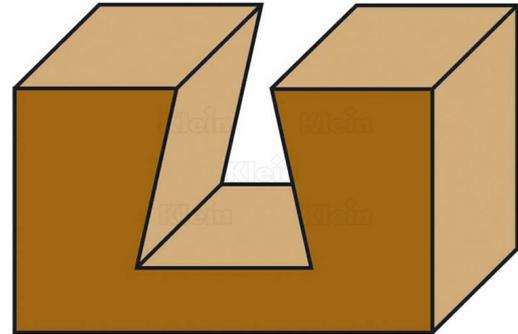
This bit is made specifically for machining dovetail joints. Dovetail joints are classic, but extremely strong, mechanical connections to be used in general woodworking. Use these joints to construct cabinet drawers, coffins, cases, or other types of furniture. Thanks to the hard metal (carbide) cutting edges, a clean and accurate result of all your milling and woodworking projects is guaranteed.
