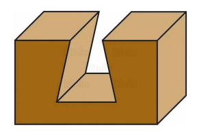
This bit is made specifically for machining dovetail joints. Dovetail joints are classic, but extremely strong, mechanical connections to be used in general woodworking. Use these joints to construct cabinet drawers, coffins, cases, or other types of furniture. Thanks to the hard metal (carbide) cutting edges, a clean and accurate result of all your milling and woodworking projects is guaranteed.
