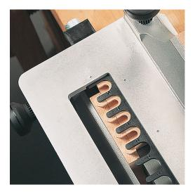
This bit is made specifically for machining dovetail joints. Dovetail joints are classic, but extremely strong, mechanical connections to be used in general woodworking. Use these joints to construct cabinet drawers, coffins, cases, or other types of furniture. Thanks to the hard metal (carbide) cutting edges, a clean and accurate result of all your milling and woodworking projects is guaranteed.
