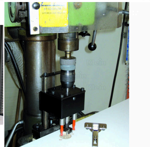
The central bit must have right hand rotation, the lateral bits have left hand rotation
