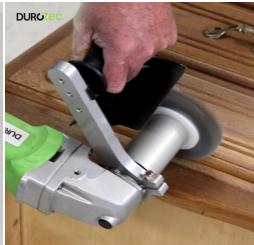
DURONYL nylon brush for texturing wooden surfaces. The characteristic wood structure is brought to the fore by working with the brush. The brushes mainly remove the softer wood of the more recent annual rings and leave the harder wood of the older annual rings intact. Brushed wooden surfaces are used, among other things, in the manufacture of rustic furniture, the furnishing of rustic cafés and restaurants (wall and ceiling coverings) or for beams.
