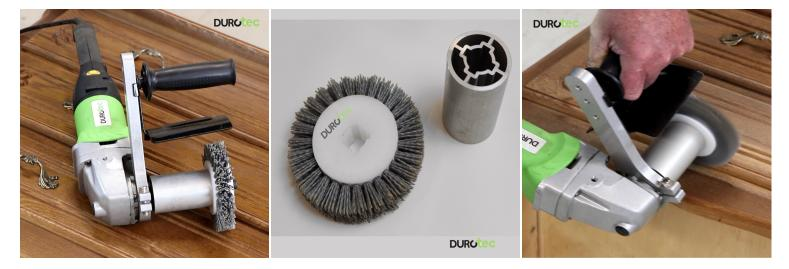
DURONYL nylon brush for texturing wooden surfaces. The characteristic wood structure is brought to the fore by working with the brush. The brushes mainly remove the softer wood of the more recent annual rings and leave the harder wood of the older annual rings intact. Brushed wooden surfaces are used, among other things, in the manufacture of rustic furniture, the furnishing of rustic cafés and restaurants (wall and ceiling coverings) or for beams.
