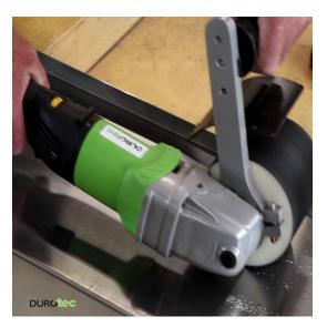
Polishing brush for polishing stainless steel, metal, lacquer, etc. Slat structure prevents the felt from burning.
