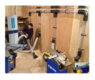
Complete set of tubes and accessories for wall mounting in workshop. This wall kit is ideal for small workshops: with one vacuum cleaner, dust extraction is provided to each machine.
