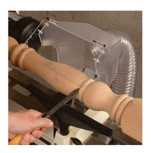
Transparant dust hood with outlet Ø100mm to be used with the Air Flux dust extractors. The size of the dust cap mouth is 200x200mm. With flap.
