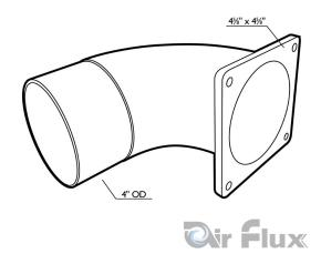
Elbow piece angle 90° and diameter 100mm to be used with the Air Flux dust extractors.
