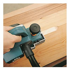
Professional, powerful Virutex chamfering planer with a base plate with a V-profile of 90°. This is why the CE89E is perfectly suited for chamfering work on all your projects. Thanks to its high power, this planer can make a chamfer of up to 25mm width in a single passage. As standard, the unit is equipped with a set of reversible blades in high-quality carbide (widia). After replacement, the blades do not need to be re-adjusted. The shavings are ejected through the exhaust on the right side.
