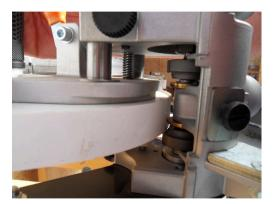
This trimmer is a time-saving solution for milling both the top and bottom of straight and round edges, without having to turn your panel over.
