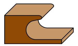
These router bits allow to create integrated pulls into drawers or doors. Thanks to the curvature of the bit, it provides positive grips and easy edge on the fingers. The Sistemi Klein finger grip bit is perfect for those who want to produce contemporary cabinet doors or drawers. Because the router bit removes large amounts of material while working, it is recommended that you keep your hands as far away from the working bit as possible.
