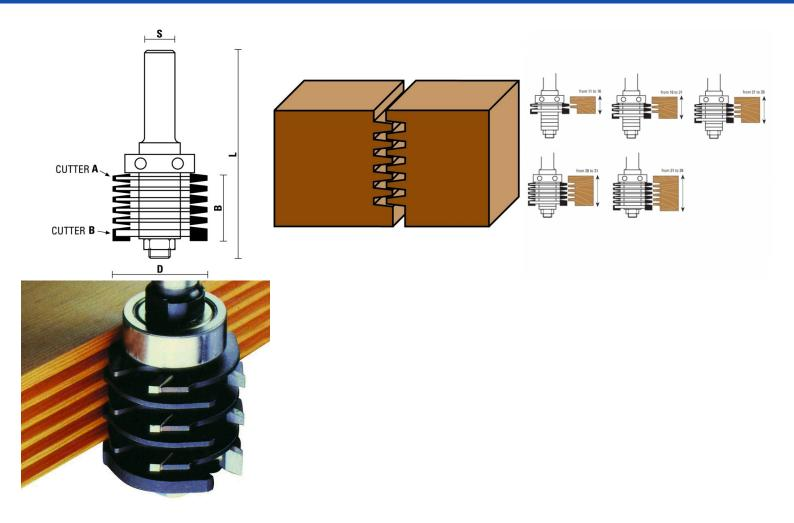
The Klein Finger-Jointer is an assembly of six high-quality carbide tipped finger slot cutters. The minimum thickness is 11mm with the one-finger slot cutter; the maximum thickness is 36 mm with the five-finger assembly. The appropriate assembly is chosen according to the wood thicknes. Using this finger joint assembly will greatly strengthen the joint significantly through extending the glue line threefold.
