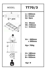
The TT70/3 is a foldable, height-adjustable roller support on ball bearings.
