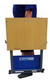
Compact work table that can be adjusted in height between 720 mm and 1150 mm. Very easy to store thanks to the foldable worktop (584x508mm). Maximum load capacity 80kg.
