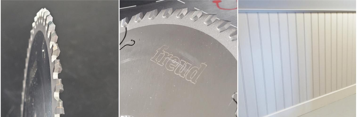
This V-groove saw blade can be used on most plunge saws (Ø 160 mm, bore 20 mm) and, with its 48 teeth, ensures a perfect finish of your V-groove on your panels, doors, etc. The teeth of this saw blade have been ground in a V-shape to make panelling easy and fast using your plunge saw.
