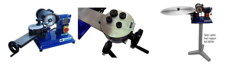
For sharpening saw blades with a diameter between 80mm and 700mm. Equipped with a 250W diamond disc and induction motor. The saw blade attachment has an adapter for blades with bore 20, 22, 25 or 30mm. With this one machine you can therefore grind a huge variety of saw blades yourself. Extremely suitable for our saw blades in chromium-vanadium but can also be used for saw blades with carbide (widia) teeth.
