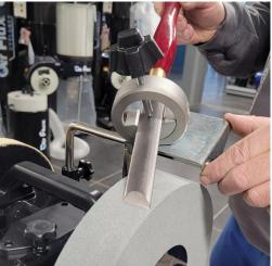
The 50K sharpening attachment for turning chisels is the solution for woodturners looking for an easy way to keep their chisels sharp. Designed for use with the wet grinder, this jig offers a quick and precise way to sharpen your beveled and hollow chisels.
