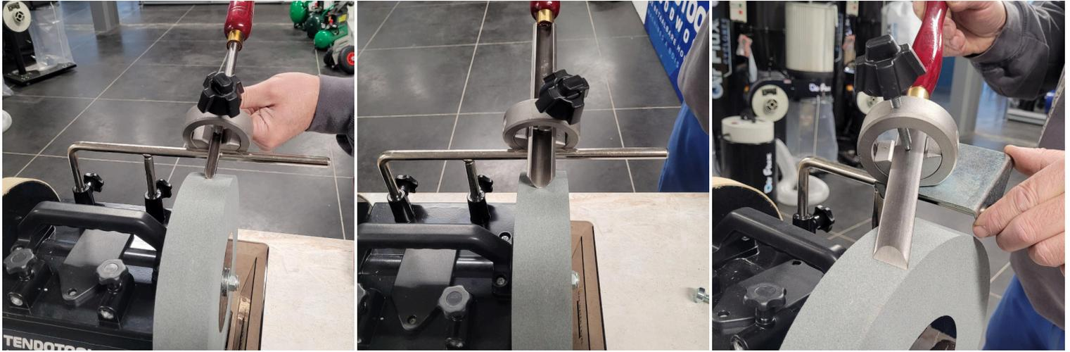
The 50K sharpening attachment for turning chisels is the solution for woodturners looking for an easy way to keep their chisels sharp. Designed for use with the wet grinder, this jig offers a quick and precise way to sharpen your beveled and hollow chisels.
