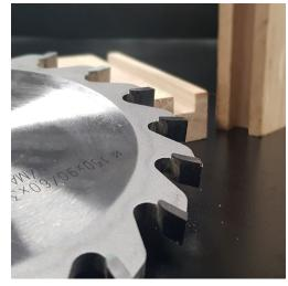
Grooving saw blade with flat (FZ) tungsten teeth to be used for cutting grooves in hardwood, softwood, timber wood, and plastic coated panel. The sawing blades have a bore of 30mm and are ideally suited for use on all spindle moulding machines or sawing tables.
