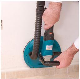
This sander from Virutex is ideal for painters and plasterers. Thanks to its low weight and ergonomic design, you can work quickly, efficiently and without fatigue. Equipped with electronic speed control, allowing optimum adaptation to the surface to be machined and to the grain of the abrasive used. Quick connection for the extraction system by means of a bayonet connection. It is possible to disassemble part of the sanding disc in order to sand hard-to-reach areas.
