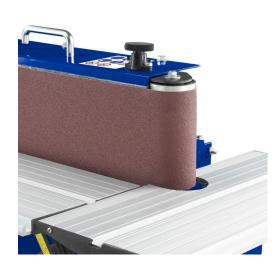
The TT2010 is a compact, versatile sander. It is equipped with a 2010 x 153 mm sanding belt, a contour table for circular sanding and an extraction outlet. The belt can be placed both horizontally and vertically. The aluminum work tables can both be tilted at an angle of up to 45°. The unbeatable price-to-benefit ratio makes this the ideal model for craftsmen. The graphite coating on the sanding table increases the sliding capcity of the sanding belt
