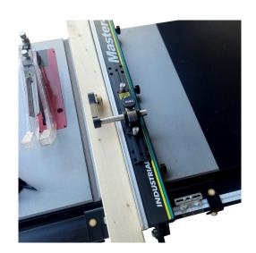
With the Precision Stock Guides, you don't have to struggle to hold plates or beams while pushing through on the saw - and router table. The rollers pull your workpiece tightly into place against the guide and your work table. You will cut more safely, easily and precisely while keeping your workpiece in place at all times.
