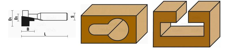
This router bit with one flint has been specially made for making keyholes (smaller T-slots) in most types of wood. The router bit in high-quality carbide (widia) guarantees you a perfect finish for all your projects. Use the plunge tip for the first working step.
