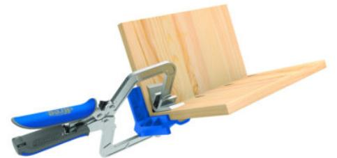
With the Kreg Automaxx angle clamp you simply and powerfully clamp 90° angle connections. Due to the Automaxx transmission in the handle, the clamping force is always optimal and the workpiece is securely clamped. There is a wheel in the handle to adjust the power transmission; heavier or lighter.
