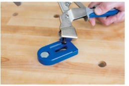
Kreg Automaxx quick release clamp for clamping a workpiece with a maximum reach of 88 mm (3 1/2"). You place the clamp in the adapter so that you can clamp it down on the workbench like a hold-down. The adapter has a connection that is suitable for 19 mm (3/4") and 20 mm (3/8") holes.
