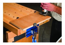
Four nylon bench hooks (so-called "bench dogs") from Kreg with rubber non-slip caps. Suitable for all workbenches with Ø 19 mm holes. The 'dogs' can be used both horizontally and vertically.
