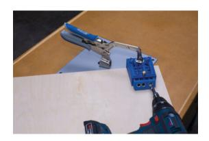
This handy kit consists of a 76 mm Kreg® bench clamp and a bench clamp foot. The clamp is equipped with Kreg Automaxx® technology, so all you have to do is attach the base to your work surface, apply the clamp and press the handles of the clamp. The clamp adapts to the thickness of the workpiece, up to a maximum of 89 mm.
