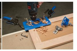
The Kreg drilling jig for hinges is a special drilling jig for the simple installation of concealed (kitchen) cabinet hinges. The placement of these hinges requires precision, otherwise you will be looking at crooked (kitchen) cabinets for years.
