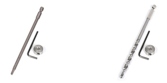
The Deck Jig<sup>™</sup> drill and screw bit are made of hardened steel and have hexagonal shanks that are compatible with Quick-Change. Both the drill bit and the screw bit are designed exclusively for the Kreg® Deck Jig<sup>™</sup> and come with a stop ring and hex key to better control the drilling and screwing depth.
