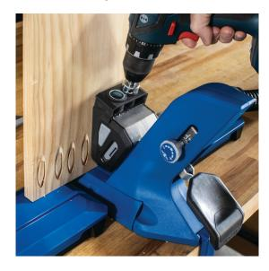
The Kreg Pocket-Hole Jig 720 and the Kreg Pocket-Hole Jig 720 Pro are compatible with the Kreg KPHA740 dowel drilling jig. With this dowel drill, you can drill your own dowels to suit your project.
