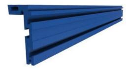
The Heavy-Duty Trak is an 'L' shaped, anodised aluminium extrusion that is extremely straight and ideal for heavy-duty commercial applications. This Trak contains four T-slots that accommodate the head of a standard 1/4" (6 mm) hex bolt. A 13mm (1/2") countersunk notch runs along the top and front of the Trak for easy attachment of an adhesive tape measure (sold separately).
