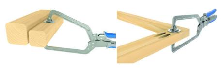
The metal quick-release clamp of Kreg has a clamping capacity of 152 mm. The clamp has large clamping surfaces to prevent surface damage. The clamp automatically adapts to any material thickness and maintains a constant clamping pressure thanks to the Automaxx technology in the handle. Compatible with Kreg Jig®, Kreg drilling guide foot and Kreg Jig® R3.
