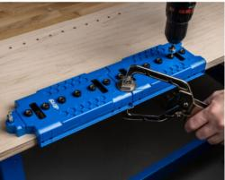
Add perfectly placed line drillings to your projects with the Kreg Shelf Pin Jig. The hardened steel drill guides ensure precision for flat, non-rolling shelves. The template comes with a 5mm brad-point drill bit. The drill guides are centred at a standard distance of 32 mm and are guaranteed for life.
