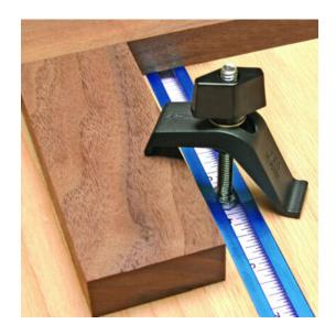
The Mini-Trak can be used to make numerous types of jigs and clamps for woodworking, such as tapered jigs and cut-off sleds. This adaptation of our popular Traks has a T-slot into which the head of a standard 6 mm hex bolt fits. A hole is provided every 10 centimetres for screwing on the profile.
