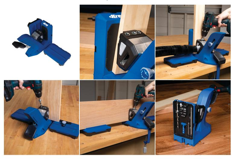
The Kreg Pocket-Hole Jig 720 Pro is the professional, fast and efficient connection system with premium accessories. With this system you can make very strong pocket holes in materials with a minimum thickness of 13 mm (1/2") and a maximum thickness of 38 mm (1 1/2").
