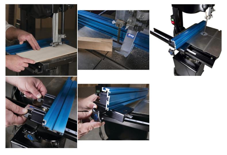
Most bandsaw blades do not run perfectly perpendicular to the front of the table. There is always just a little bit of "drift" that prevents you from getting precise cuts, even if you use a fence.
