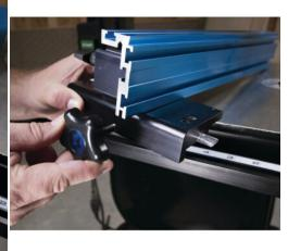
Most bandsaw blades do not run perfectly perpendicular to the front of the table. There is always just a little bit of "drift" that prevents you from getting precise cuts, even if you use a fence.
