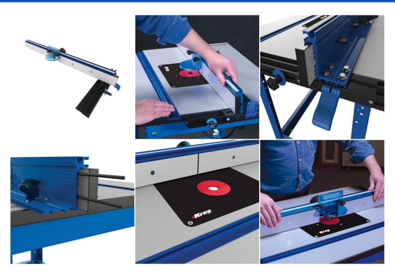
This guide rail made of anodised aluminium is equipped with a T-shaped adjustment system that keeps the rail always parallel to the mitre gauge groove. The guide rail is easy to adjust and is held firmly in place with a double locking mechanism, namely a lever on the input side and a quarter-turn knob on the output side, so that the rail does not bend.
