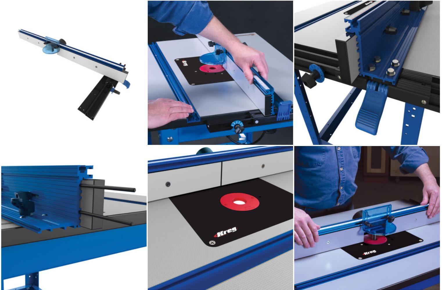
This guide rail made of anodised aluminium is equipped with a T-shaped adjustment system that keeps the rail always parallel to the mitre gauge groove. The guide rail is easy to adjust and is held firmly in place with a double locking mechanism, namely a lever on the input side and a quarter-turn knob on the output side, so that the rail does not bend.
