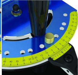
The Kreg KMS7102 precision miter gauge is adjustable from -45° to 45°. It is equipped with preset angles at 0°, 10°, 22.5°, 30° and 45°. The brass pin makes it easy to switch between these angles. In addition to these preset angles, the mitre stop is adjustable with 0.1° precision. Markings are indicated per 1°. The supplied guide has a length of 610 mm and has a reversible stop.
