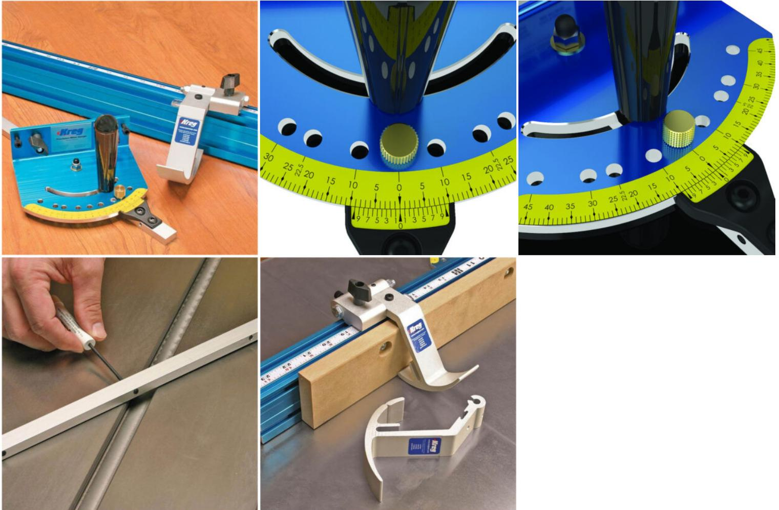
The Kreg KMS7102 precision miter gauge is adjustable from  $-45^{\circ}$  to  $45^{\circ}$ . It is equipped with preset angles at  $0^{\circ}$ ,  $10^{\circ}$ ,  $22.5^{\circ}$ ,  $30^{\circ}$  and  $45^{\circ}$ . The brass pin makes it easy to switch between these angles. In addition to these preset angles, the mitre stop is adjustable with  $0.1^{\circ}$  precision. Markings are indicated per  $1^{\circ}$ . The supplied guide has a length of 610 mm and has a reversible stop.
