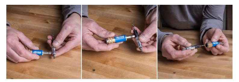
The Kreg Quick-Flip allows you to use Kreg screws for a variety of strong, simple connections - all with a single tool. You pre-drill on one side, then turn the Quick-Flip around and drill a Kreg screw in smoothly. Thanks to the double action of this tool, you can quickly make connections with Kreg screws in many different applications.
