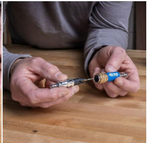
The Kreg Quick-Flip allows you to use Kreg screws for a variety of strong, simple connections - all with a single tool. You pre-drill on one side, then turn the Quick-Flip around and drill a Kreg screw in smoothly. Thanks to the double action of this tool, you can quickly make connections with Kreg screws in many different applications.
