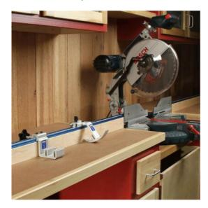
The Kreg Top Trak is an aluminium track that can be easily attached to an existing fence. Due to the L-shape, the track fits well to the existing fence. Drill Ø 3 mm holes on the back and attach with the screws provided.
