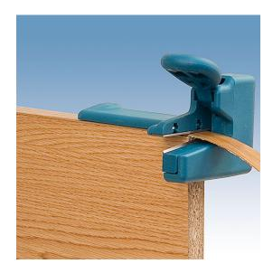
Manual end trimmer for PVC, melamine, polyester, veneer, etc... up to a maximum thickness of 0.6mm. The maximum width to cut edge bands is 54mm. The trimmer makes a perfect, clean cut at all corners of the board. Equipped with reversible and replaceable blades.
